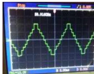
Figure 4.9. Output Voltage of MLI
